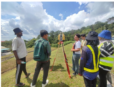
Group A collecting the point cloud data for slope modelling.
